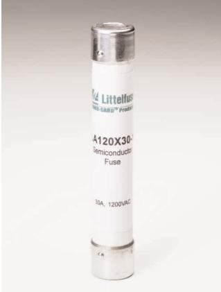
Littelfuse's LA120X semiconductor protection fuses, rated 1/2 through 30A, 1200 VAC are popular for use in traction drive auxiliary circuits and similar applications. LA120X fuses are also suitable for use on 1000VDC auxiliary circuits with low time constants.
